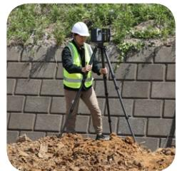
Despite its high performance, the compact and lightweight body (4.4 kg) and the quick-release mechanism that allows easy attachment and detachment from the tripod providing excellent mobility. Even in environments where frequent repositioning is required, shifting the scanner is quick and easy.
